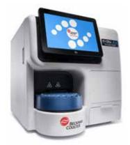
The Vi-CELL BLU automates the widely accepted trypan blue dye exclusion method for cell viability that has historically been performed with a light microscope, pipette, and a hemacytometer. This makes it perfect for large-to small-scale cell viability/counting applications in many fields including biopharma and academia.
